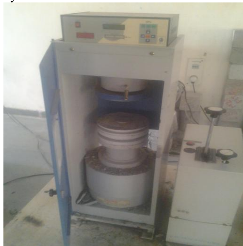
Fig. 1. shows compressive testing machine used to determine the compressive strength of plain concrete. The compressive strength of specimen will be calculated by following formula,
