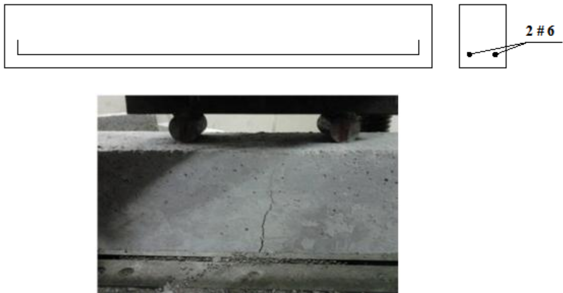
Fig 3 Beam specimen under UTM with four point loading
