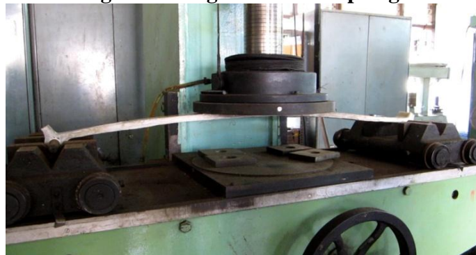
Fig. 6: Testing of E-glass/Epoxy Composite leaf spring.
