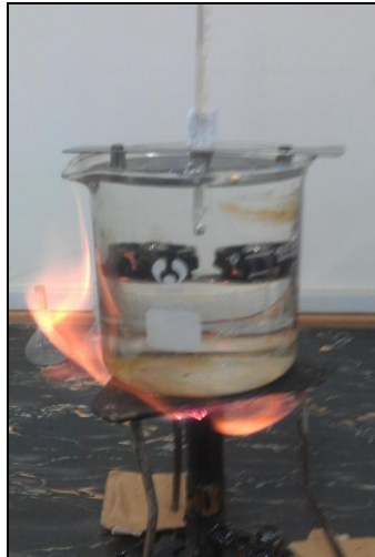
Figure 3: Apparatus for Determining Softening Point of Asphalt
