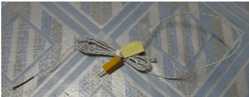
Fig 8 K-type thermocouple probe.
