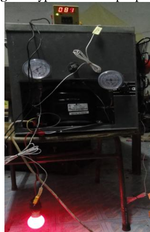
Fig 9 Refrigeration system during the experiment.
