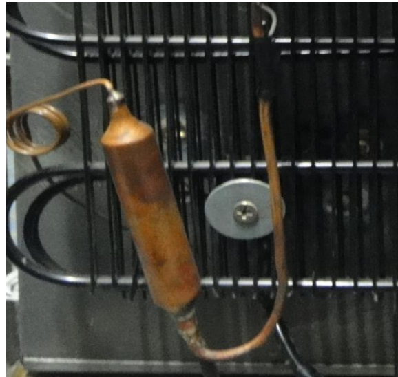
Fig 5 Filter fitted with an Expansion valve.
