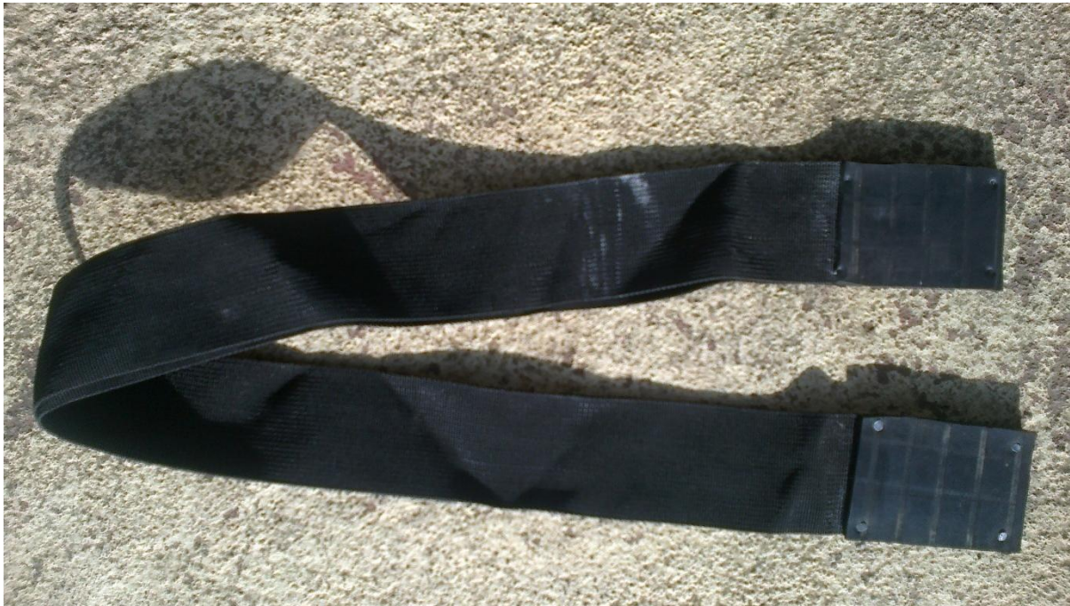
Fig. 3 Nylon belt with rubber pads used for testing.
