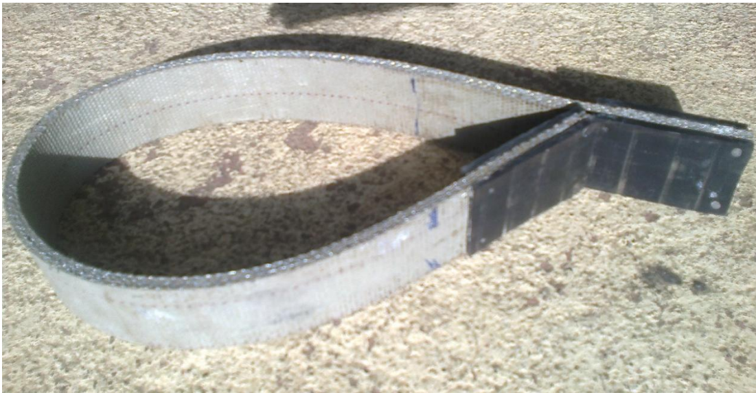
Fig. 1 Polyester belt with rubber Pads for testing
