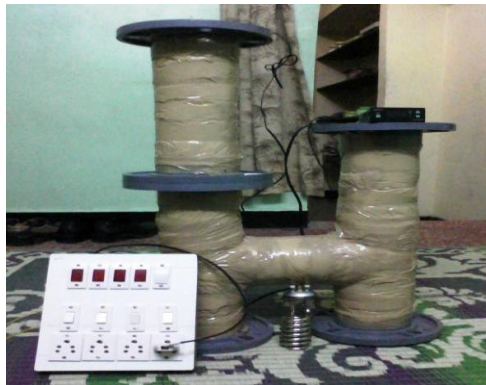
Fig.5 test rig for checking thermal conductivity of material
