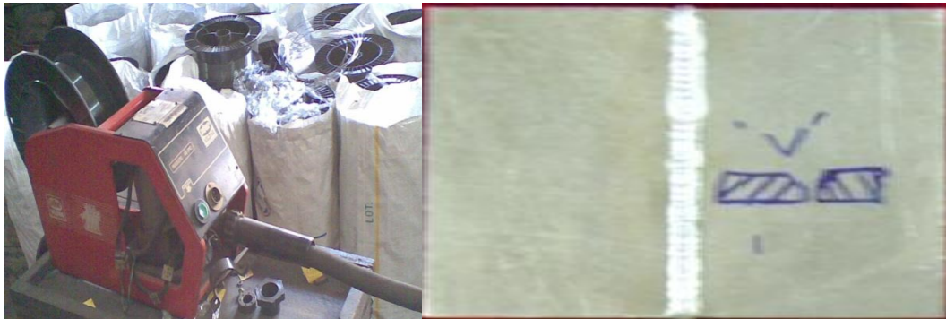
Fig .1 (a). Welding experimental set up used for GTAW Fig .1 (b). Fabricated Weldments by GTAW
