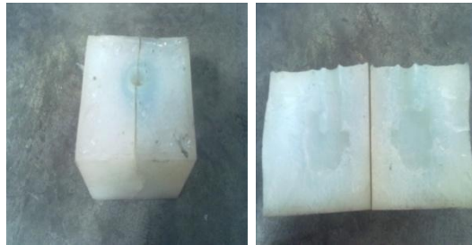
Fig. 6. Mould (cope and drag) of component 2
