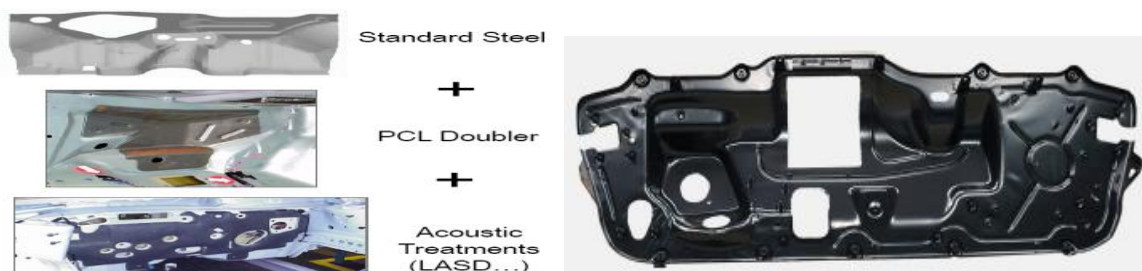
Fig.3: Conventional steel automotive dash structure & Silent Steel Dash Panel.
