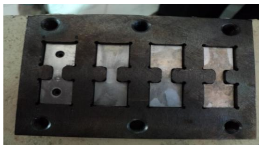
Fig. 2. Configuration of the diffusion bonding setup
