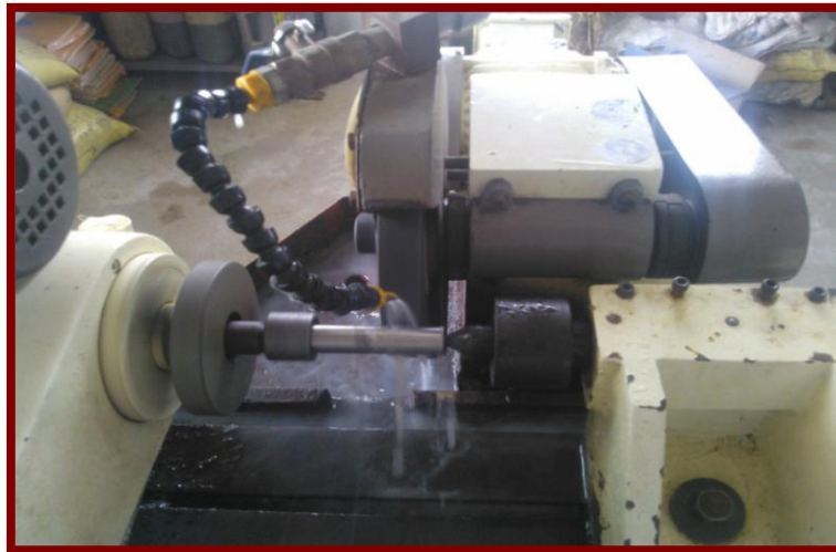
Figure 4 Cylindrical grinding machine with workpiece actual setup
