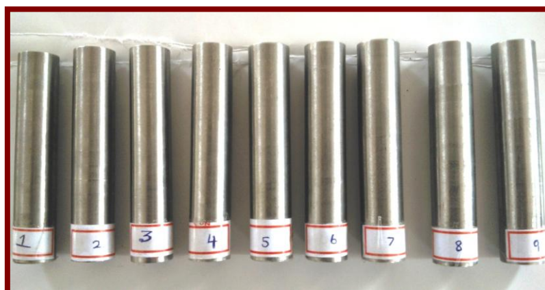
Figure 5 Actual Workpiece after Cylindrical Grinding process
