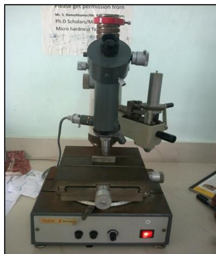
Fig 3.4.2 Vickers hardness testing machine (Zwick 3212 hardness test)
