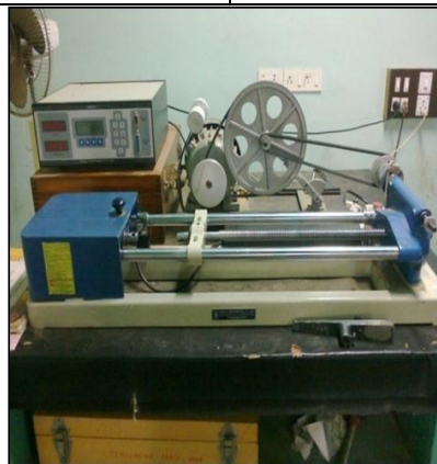
Fig 3.4.4 Tensometer (TIMER3) for tensile test
