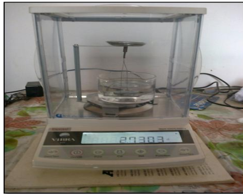
Fig.3.4.3 Density measuring instrument
