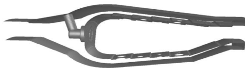
The 30 degree sector of designed stage-3 combustor
