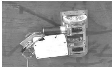
1-active magnetic wheel unit; 2-reducer; 3-motor; 4-passive magnetic-wheel unit; 5-body
