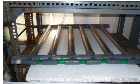
Figure 3. Assembly of heat exchanger
