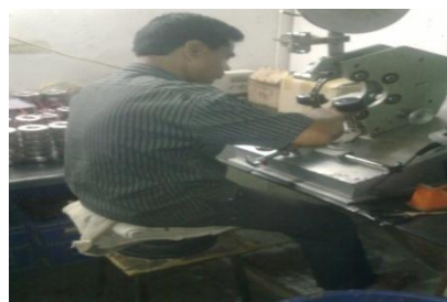
Figure1. A typical working posture adapted in order to perform Transformer winding operation.
