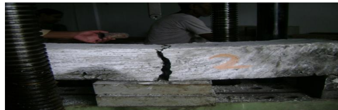
Fig4: Failure of Beam with fiber
