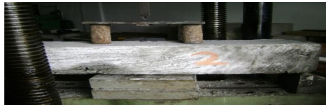
Fig3: Beam under loading with fiber
