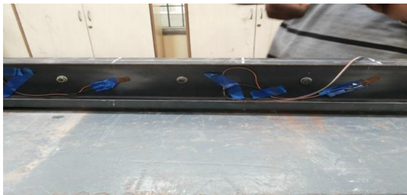
Fig 5.3.1 : Placing Strain Gauge in Beam
