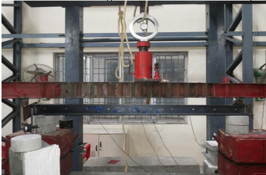
Fig 5.3.2 : Full Loading Setup
