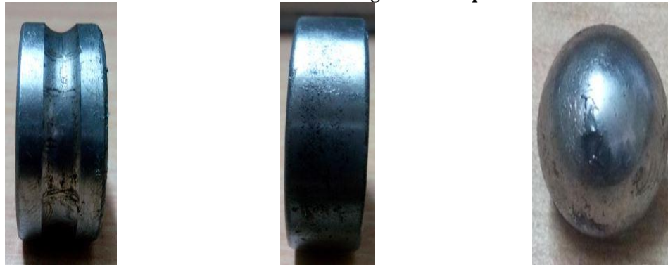
Fig. 2. Bearing With Inner Race Crack And Outer Race Crack And Corrosion Pitting
