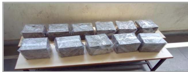
Fig1. Cubes packed in thick plastic wraps for ambient curing.
