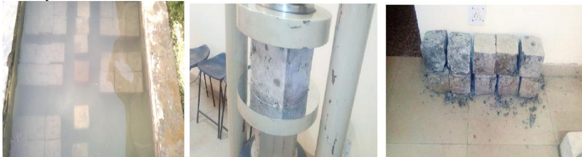
Fig.4. Procedure of compressive strength test being executed
