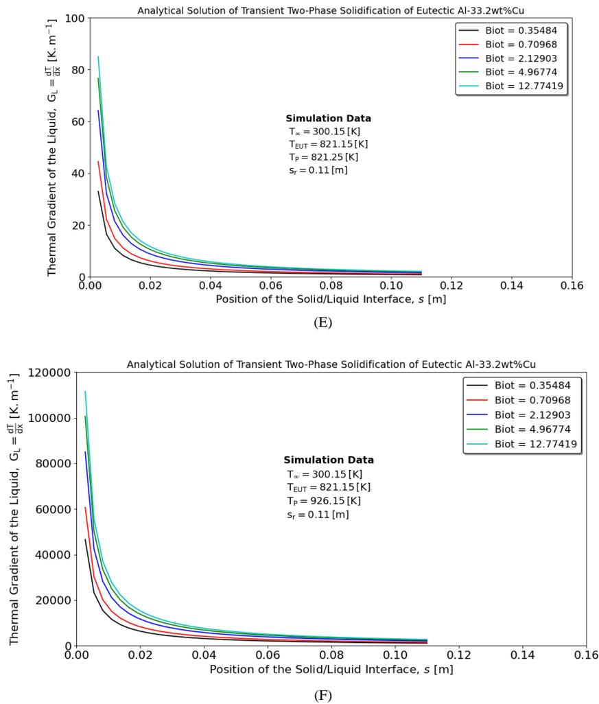
**Figure 9** Analytical solution of unidimensional solidification Al32.2wt%Cu against numerical simulation for 0.1K and 105K of melt superheat: (A) and (B) position of solid/liquid interface as a function of time, (C) and (D) temperature profiles, and, (E) and (F) thermal gradients of the liquid.
