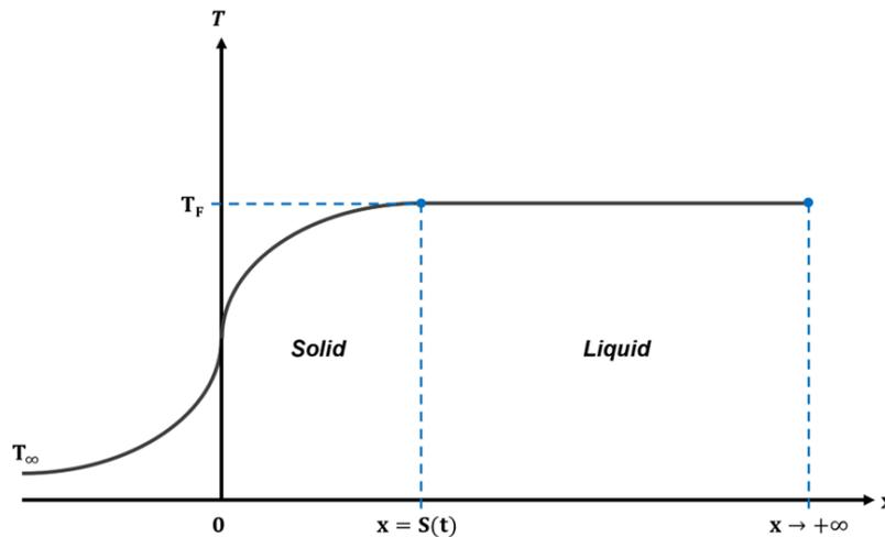
**Figure 1 Schematic representation of one-phase transient solidification.**
