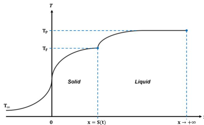
Figure 2 Schematic representation of two-phase transient solidification.
