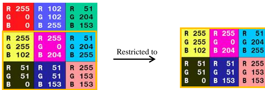
Figure 2. This figure show the restriction of 3×3 matrix of Pixels in to a of 2×3 matrix of Pixels .
