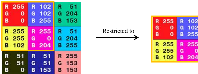
Figure 1. This figure show the restriction of 3 \times 3 matrix of Pixels in to a of 2 \times 2 matrix of Pixels .
