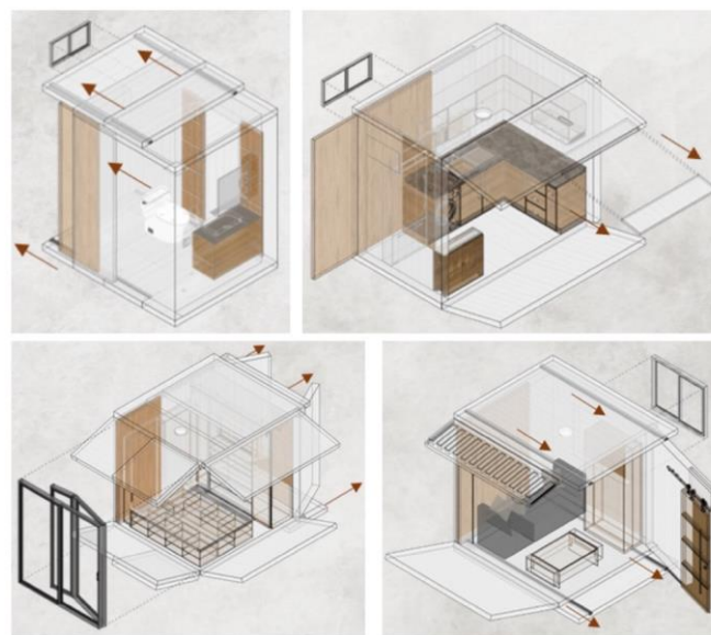
Figure 6. MODU-LOFT: Expansion of the bathroom, kitchen, bedroom and social area modules. Source: Own elaboration (2022)
