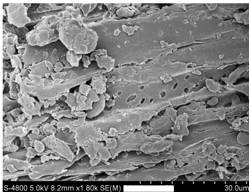
Figure 2: Scanning electron microscope image of raw tur dal husk
