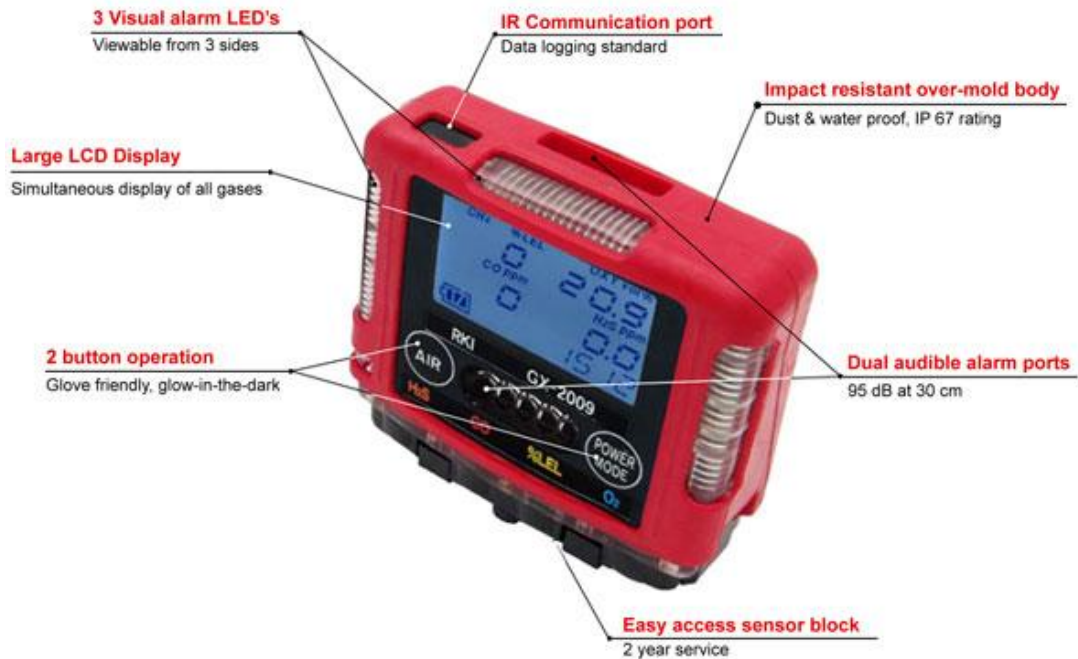
Photograph 3.5: RKI GX-2009 Multi-Gas Detector (Source: Google)
