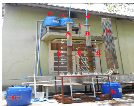
Fig. 2 Experimental set up for Rapid sand filter unit
