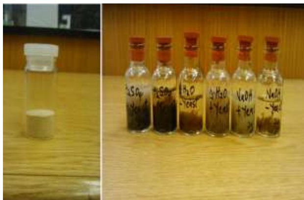
Fig 4. The activated yeast strain used for the fermentation experiment and the setup applied for the fermentation process. We had a blank for each pretreatment technique.
