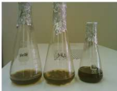
Fig 3. The color change observed after hydrolysis from different pretreatment techniques
