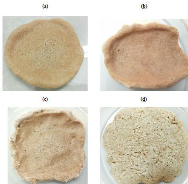
Fig.2 Natural fiber sorbent under condition of 18% sodium hydroxide, carbon disulfide 25% (a) sodium sulfate ratio 1:1.5 (b) sodium sulfate ratio 1:2 (c) sodium sulfate ratio 1:2.5 and (d) sodium sulfate ratio 1:3
