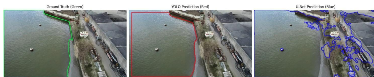
Figure 11: Water class segmentation. Ground Truth (Green), YOLOv8 Prediction (Red) and U-Net Prediction (Blue).
