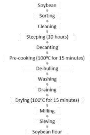
Fig. 2 Flow chart for the production of soybean flour
