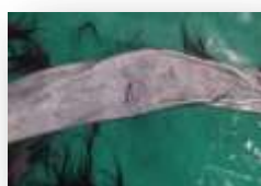
Figure 10 (a):Pretanned pelt converted from Mimosa pudicaAgNPs preserved skin in which complete removal of keratin protein
