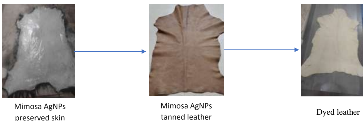
Figure 12: Mimosa pudicaAgNPs tanning process of leather.
