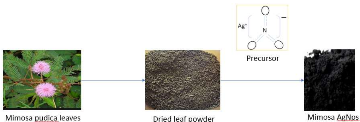
Figure 1: The synthesis of Mimosa AgNPs
