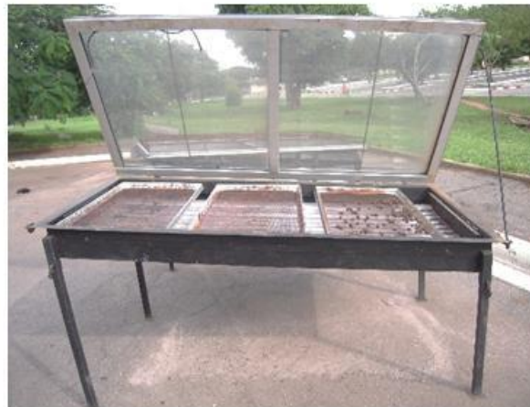
Figure no 3: Drying in a direct solardryer on a sheetmetaltray (aluzinc)
