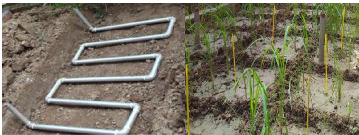
Photographs 5-6 Instrument and approaches for the elevation of soil temperature by 2 and 4°C during field study
