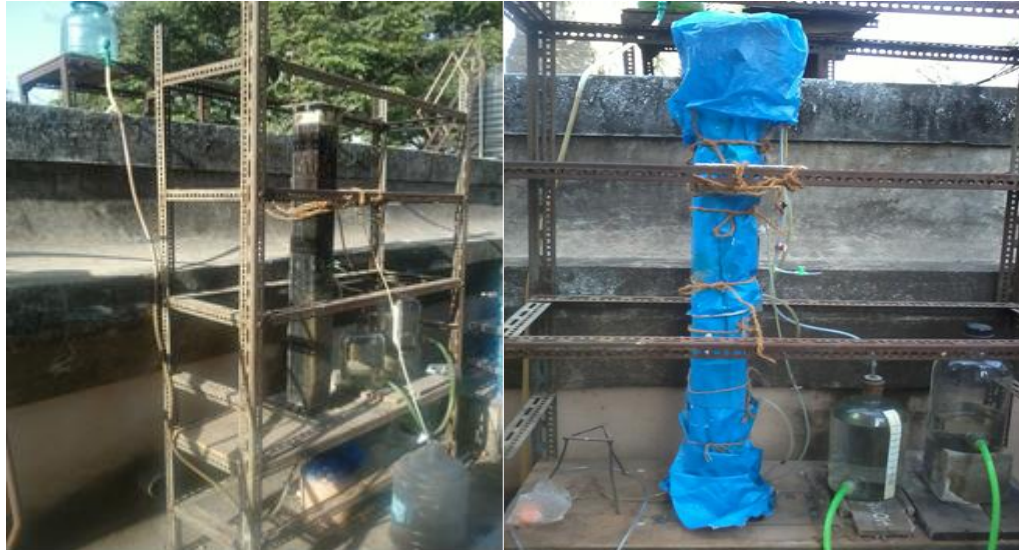
Fig No.2: Upflow Anaerobic Filter Experimental Setup & Covered with tarpaulin sheet.
