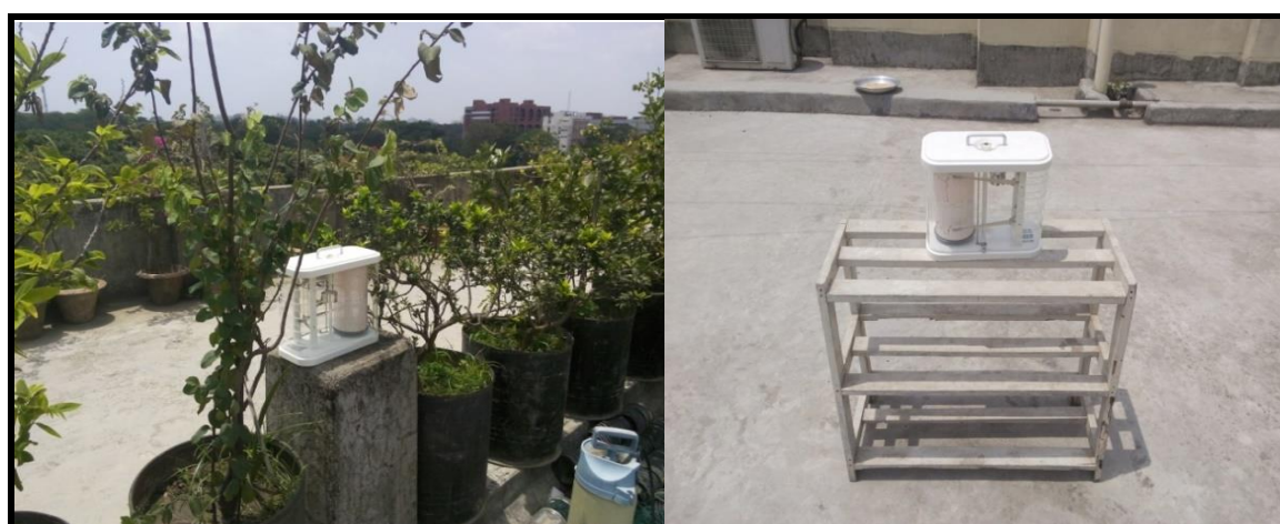
Fig 1. Thermal data collection using thermo-hygrograph in (a) roof garden and (b) bare roof
