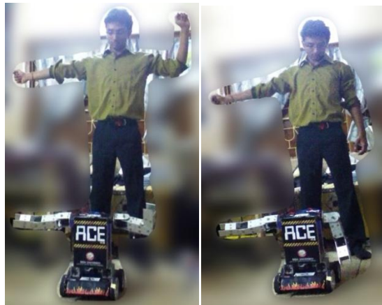
Figure7. Imitation of its human operator by ACE, the semi-humanoid robot.
