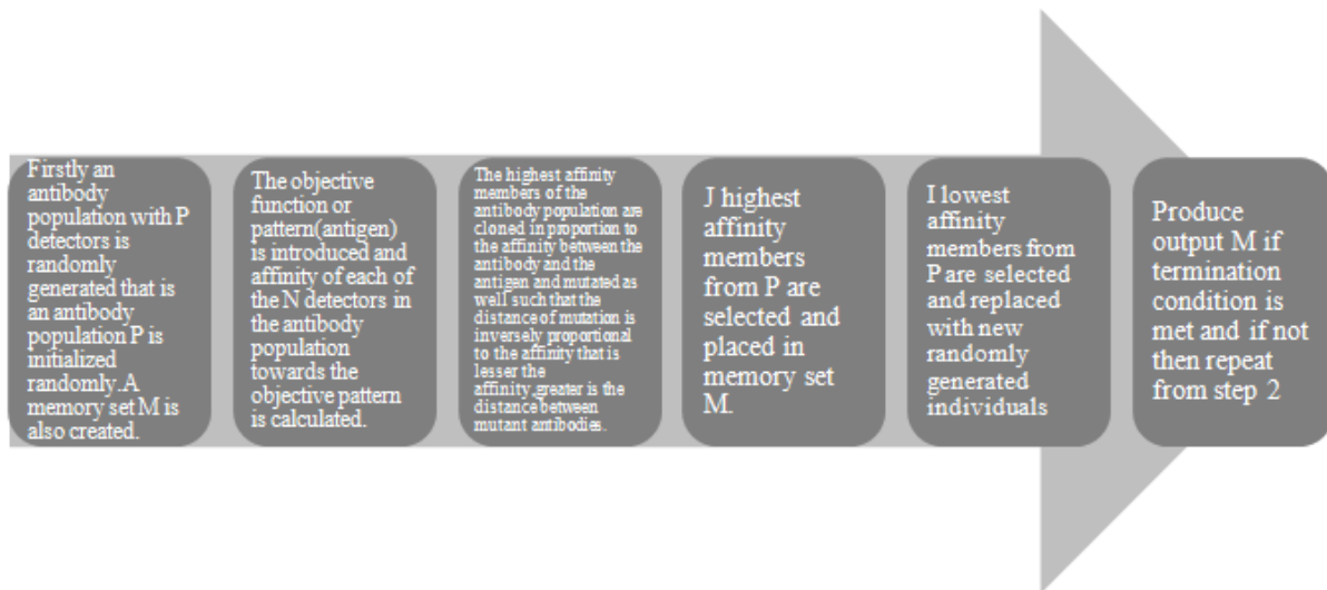
Figure 2. Clonal selection algorithm
