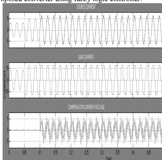
Fig:14. Simulation results for Un Balanced Non Linear Load using fuzzy controller (a) Source current. (b) Load current. (c) Inverter injected current.
