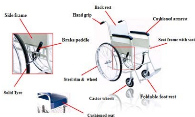
Fig. 1 Nomenclature of a rigid frame wheel chair
