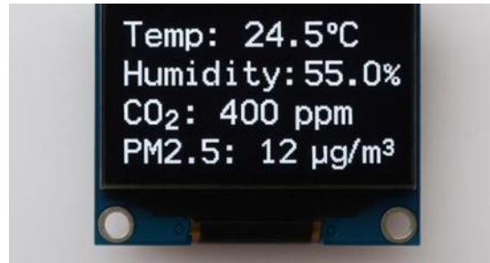
Figure 2: OLED Display during the simulation (temperature, humidity, CO 2 , PM2.5).
