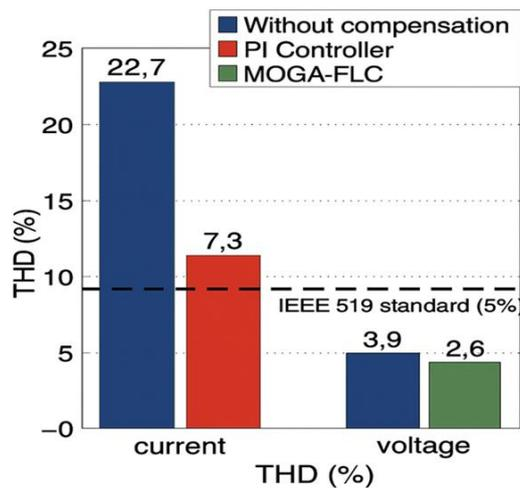
Figure 4: Power Quality and Harmonic Distortion
