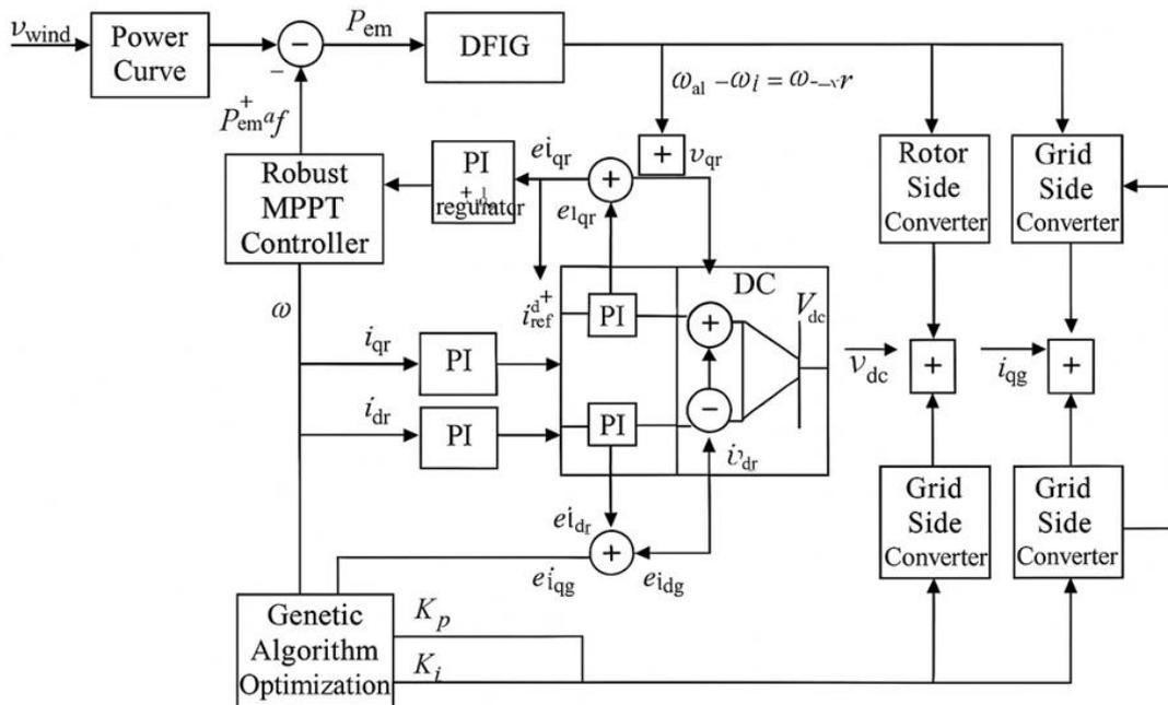
Fig. 1. The schematic of the Proposed Robust MPPT and DFIG-Based Control of Grid-Connected Wind Energy Systems Using Multi-Objective Genetic Algorithm Optimization.
