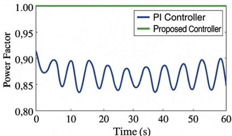
Figure 5: Reactive Power Compensation and Power Factor Improvement
