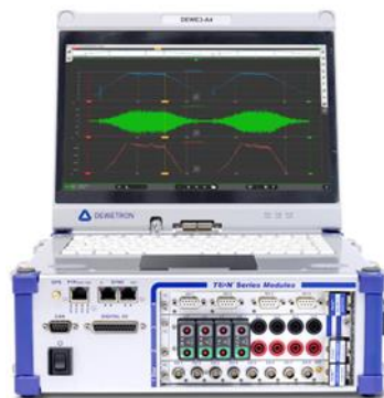
Figure 1.1: Front view of the data acquisition device DEWE3-A4 [2]
