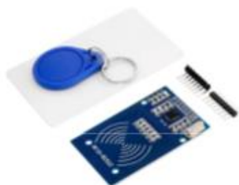
Figure 2.1: RFID reader RC522 [6]
