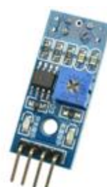
Figure 2.2: Infrared sensor TCRT5000 [7]
