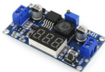
Figure 3.1: LM2596S DC-DC buck converter for GSM module [10]
