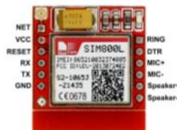
Figure 2.4: Pinning of the SIM800L GSM module [9]
