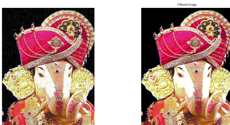
Figure 1.8: Use for Median Filter to improve corrupted Image
