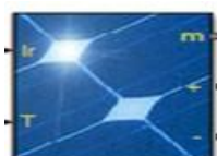
Figure 2: Simulink block of a Solar Photovoltaic Module
