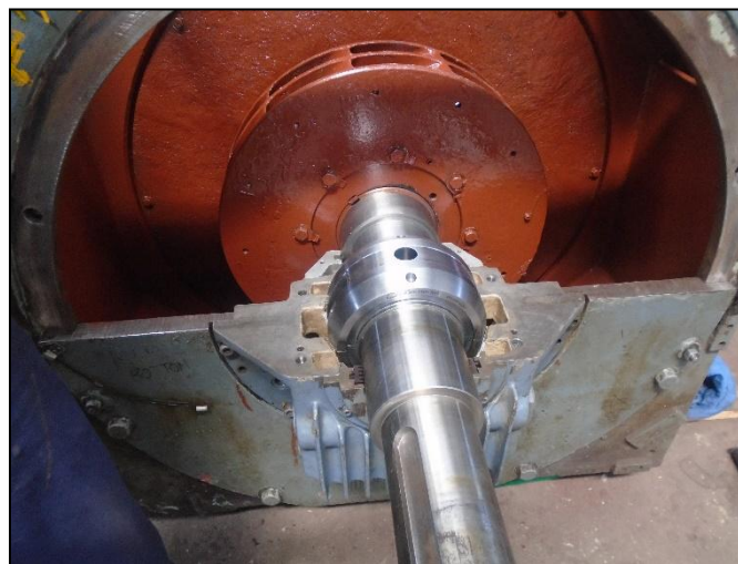
Fig. 6: Bearing Housing Assembly
