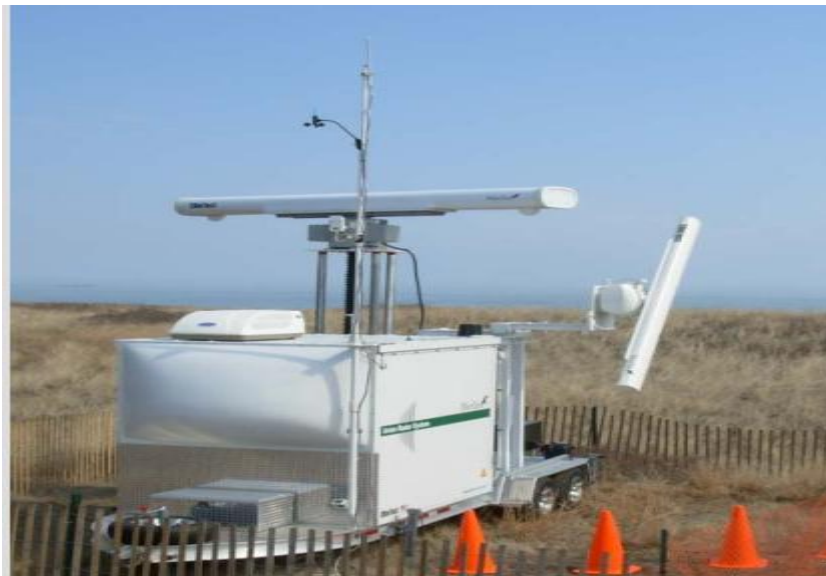
Figure 10 shows an illustration depicting the fencing of the radar to minimize wave clutter. (iv). Atmospheric Effects
