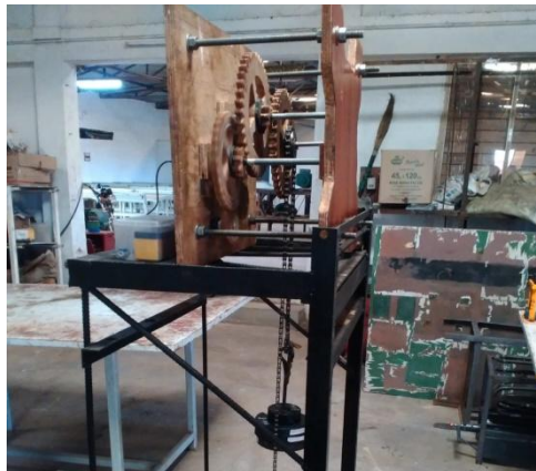
Figure 3: Power generation system using gravity
