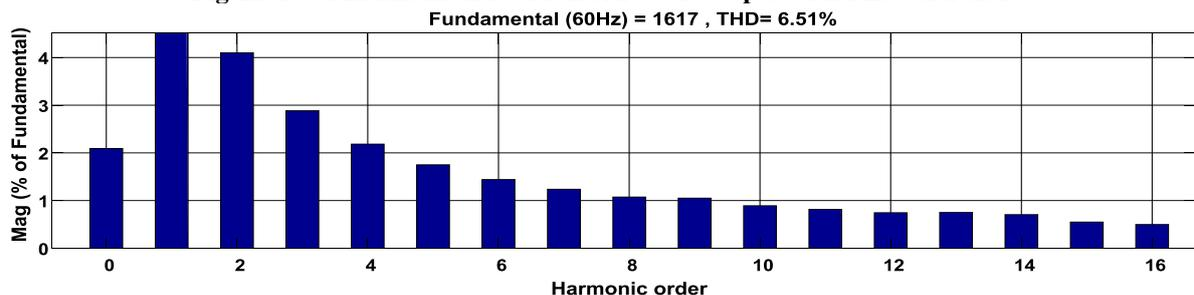
Fig.13 Total Harmonic Distortion of Power Output with FLC controller
