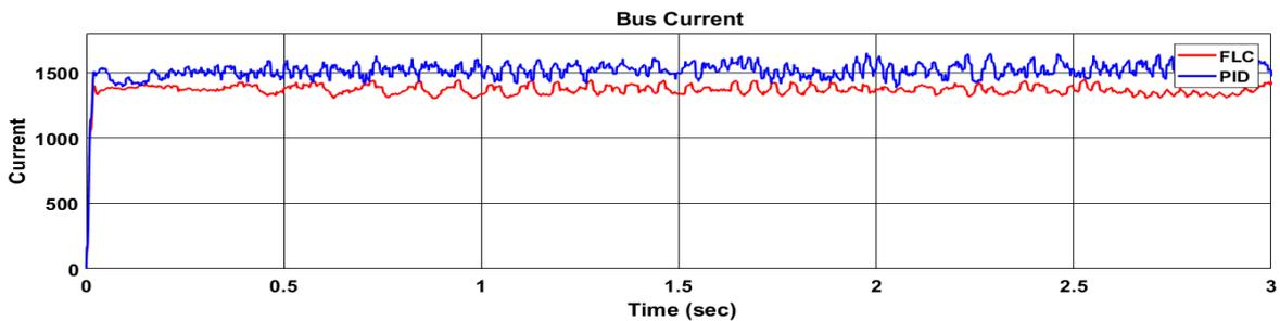
Fig 15. Comparison of bus Current of UPQC using FLC and PID controller
