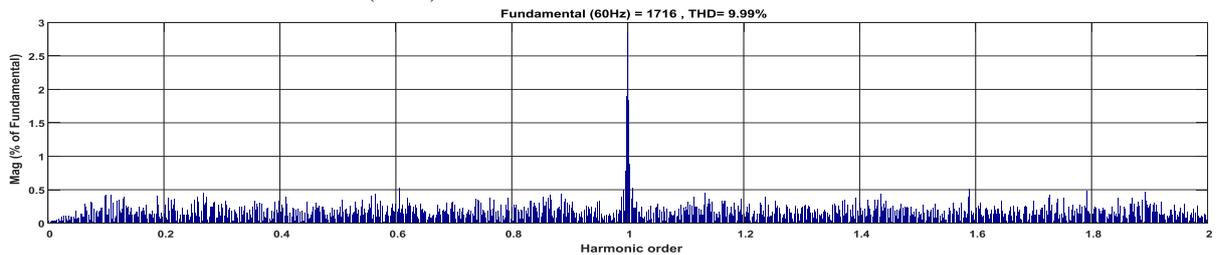
Fig.12. Total Harmonic Distortion of Power Output with PID controller
