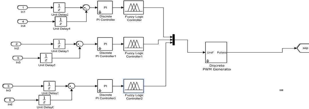
Fig. 10. Shunt controller with fuzzy logic controller for UPQC
