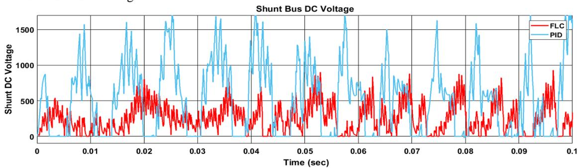
**Fig 17 Comparison of Shunt bus DC Voltage of UPQC using FLC and PID controller**
