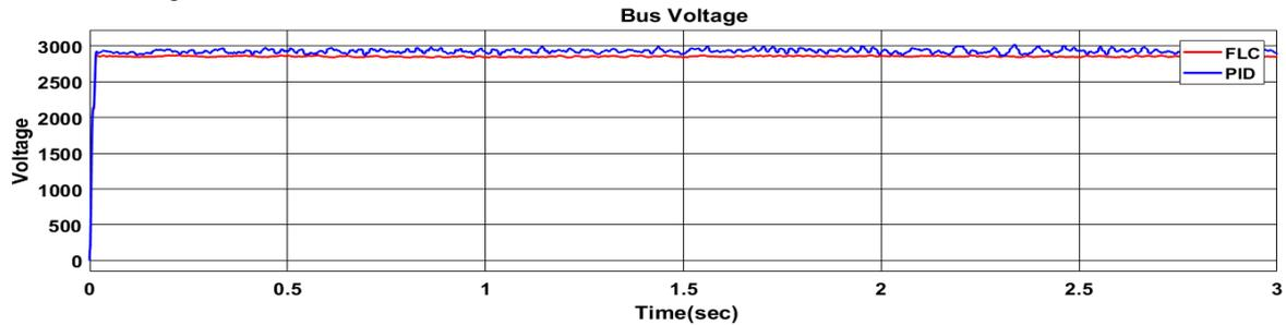
Fig 14. Comparison of bus Voltage of UPQC using FLC and PID controller
