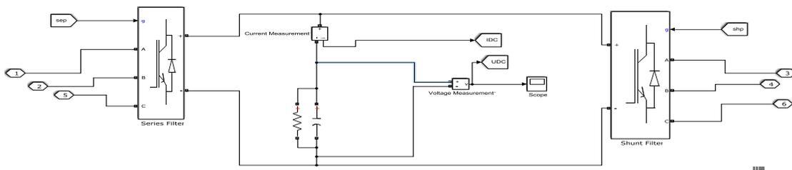
Fig. 8. MATLAB model for UPQC with series and shunt converters
