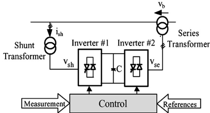
Fig.2 Block Diagram of UPFC
