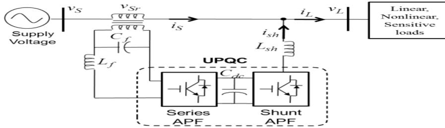
Fig.5 Block diagram of UPQC
