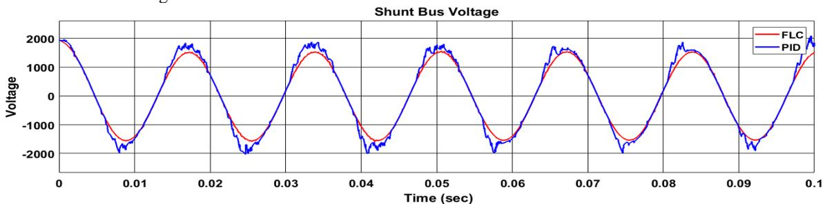
Fig 16 Comparison of Shunt Bus Voltage of UPQC using FLC and PID controller
