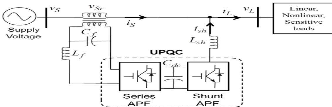
Fig.4 Block Diagram of UPQC
