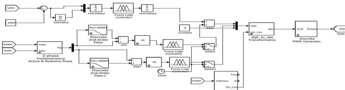
Fig. 11 Series controller with fuzzy logic controller for UPQC
