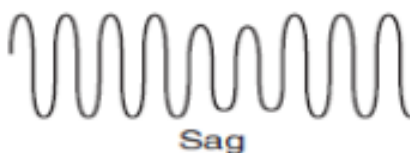
Fig.3 Sag in transmission line voltage waveform
